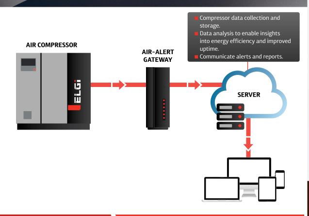
Air~Alert acquires operational data from compressor and sends it to a dedicated, secured server. Intelligent algorithms in the server analyzes the data and enables useful insights to improve energy efficiency, uptime and remote monitoring from anywhere in the world.
